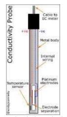
Figure 3 [7]: An electrical conductivity sensor measures the ability of a solution to conduct electricity, a property directly related to ion concentration, which the sensor measures in units of
