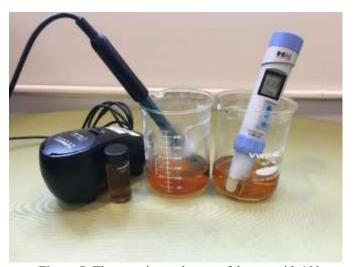
**Figure 5:** The experimental setup of the tea, with 100 mL of liquid in 2 standard beakers. The Vernier pH sensor and the Vernier turbidity sensor were both connected to the Logger Pro software on a laptop, and continuously measured data over a duration of 1 min, with a sampling frequency of 1 sample/second. The HM Digital COM-100 electrical conductivity sensor was manually inserted into the tea, and the reading, in millisiemens per meter, was recorded.
