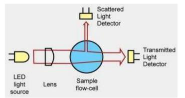
**Figure 2** [7]: A turbidity sensor measures the concentration of undissolved particles in water, by sending a light beam through the liquid, and measuring the amount of light scattered and reflected onto the sensor, in units of Nephelometric Turbidity Unit (NTU). The sensor is at a 90° angle to the light source; thus the more the reflected light the sensor receives, the higher the concentration of particles in the liquid.
