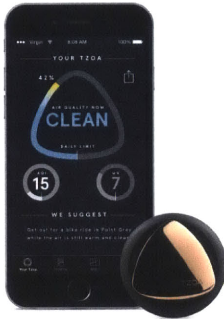
Fig. 15. TZO A, Tzoa sensor and smartphone app . From: Tzoa. "About," TZO A.com , accessed August 2015. http://tzoa.com/about-tzoa
