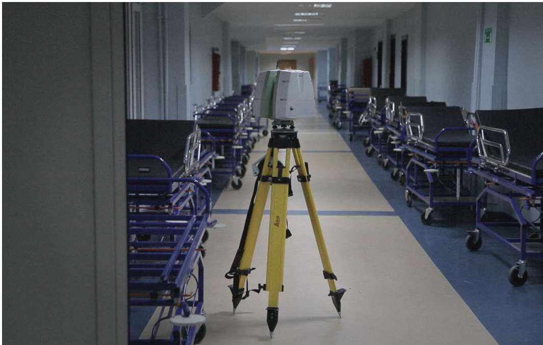
Figure 2.7: 3D laser scanner capturing the OR corridor
