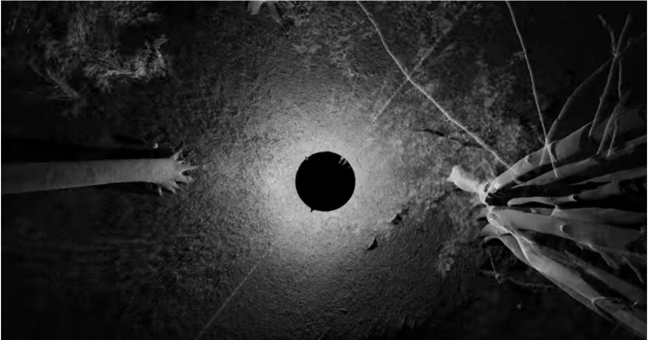
Figure 3.11: The black hole at the initial position of the body; at the original point-cloud capturing position of the laser scanner in Phantom
