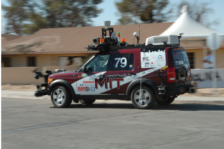
Figure 1-3: MIT's Urban Challenge vehicle. The grey cylindrical sensor at the top is a Velodyne LIDAR sensor. Below it sits a row of other LIDAR sensors and cameras. Picture credit: DARPA [DARPA, 2007].
